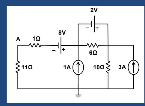
Determine the voltage V<sub>A</sub>
