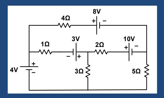
Determine the currents through 4V, 8V and 3V sources, and  $3\Omega$  resistor
