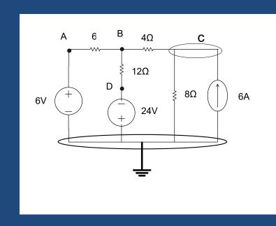
Determine the voltages V<sub>A</sub> and current I
