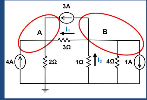
Determine the voltages  $V_A$  and  $V_B$ Note: There is a voltage source with one polarity connected to the ground
