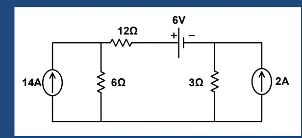
Determine the currents through  $3\Omega$  resistor
